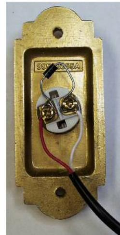
A full installation diagram complete with diode is shown on the picture to the right.
